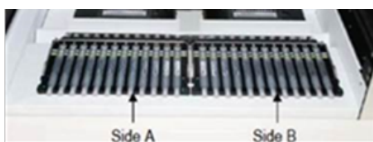
Figure 3: Load Rack(s) into the BD MAX System
