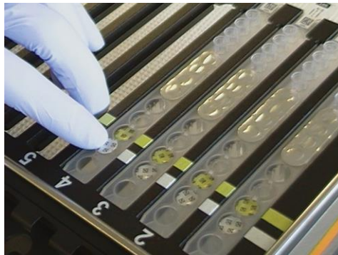
Figure 1: Snap BD MAX Check-Points CPO Extraction tubes and BD MAX Check-Points CPO Master Mix tubes into Unitized Reagent Strips
