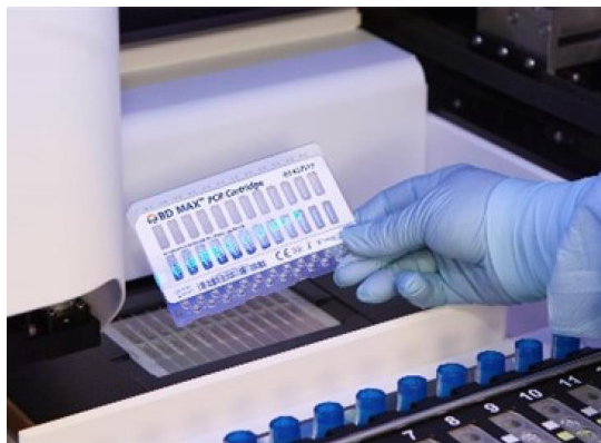
Figure 2: Load BD MAX PCR Cartridges
